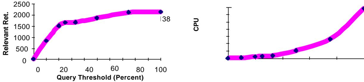
Figure 3. Relevant Retrieved and Computation Time as a Function of Query Threshold
