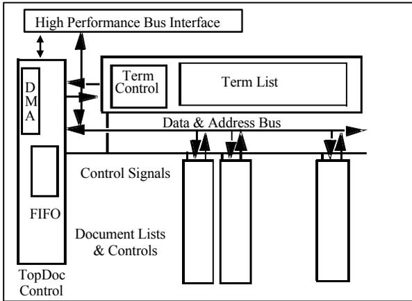
Figure 2. The HAT System Architecture
