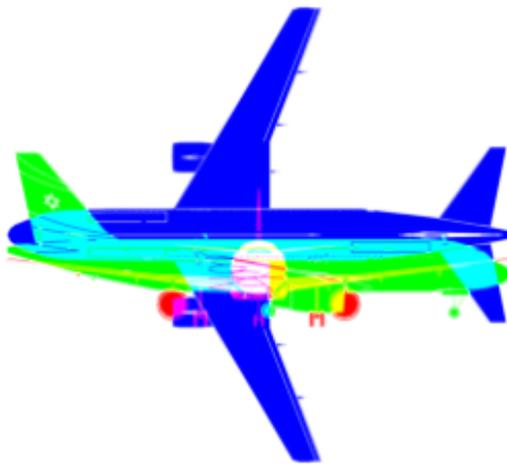
**Figure 7: Combined three-view image. The front view is in the red image plane, the left view is in the green image plane, and the top view is in the blue image plane.**
