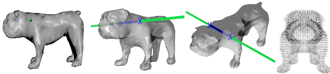
Figure 1: Sampling a point cloud from multiple images. Left: Source image with selected sampled point in green. Middle: Epipolar projections of the selected point onto orthogonal images. Right: Resulting sampled point cloud.
