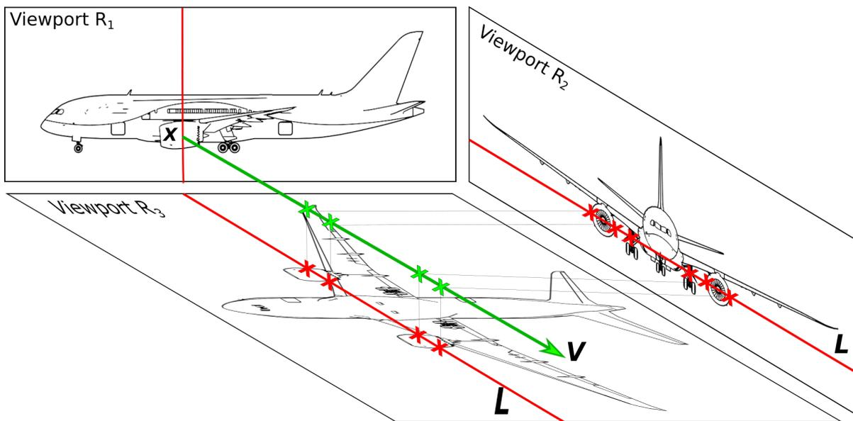
Figure 9: Projection of point  $X$  from the right side multiview image, viewpoint region  $R_5$ . The green line represents the vector projection  $L$  of  $X$ . The red lines on the front and bottom multiview images are the epipolar projections of  $L$  onto the image. The red Xs represent the intersections of the  $L$  with the image silhouette.
