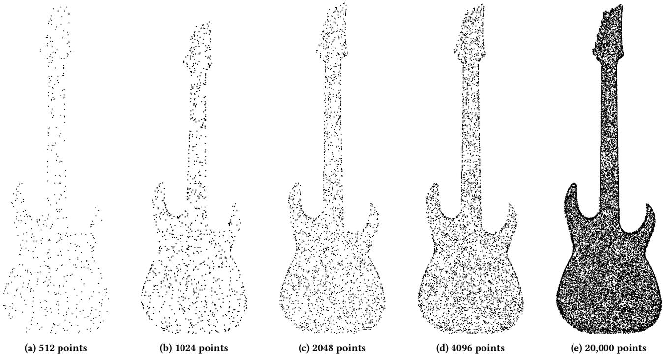
**Figure 11: Point cloud model of a guitar sampled directly from multiview images using various point densities.**
