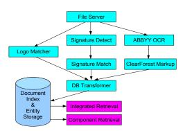
Figure 1: Architecture of the current prototype.
